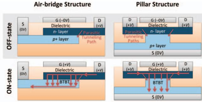
**Figure 1.** Diagram of the air-bridge and pillar structures in the OFF- and ON-states. The red arrows indicate BTBT currents. Both structures suffer from diagonal parasitic tunneling that limits OFF-state current and degrades the switching abruptness.
