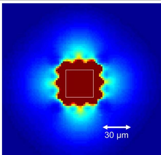
Fig. 6. Spot scan response map of the 15- $\mu$ m-pitch 4- $\mu$ m-via mini-array on test bar D5394.1, measured at 300 K.
