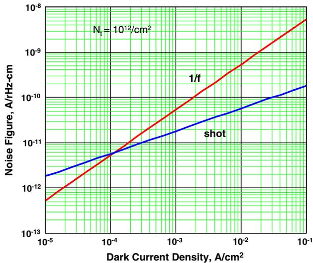
Fig. 8. Predictions of the Schiebel<sup>6</sup> model for the  $1/f$  noise for a surface trap density of  $10^{12} \text{ cm}^{-2}$ . The dark current shot noise is also shown.
