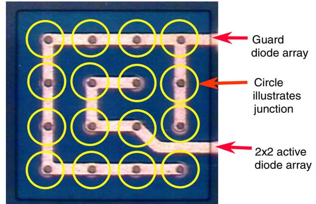
Fig. 2. HDVIP mini-array on a test bar. A test bar contains mini-arrays having different via diameters and pixel pitches.
