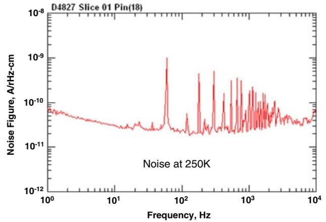
Fig. 7. Noise measured at 250 K in Test Bar D4827.1. At 1 Hz, the  $1/f$  noise is  $6 \times 10^{-11}$  A/rHz-cm.
