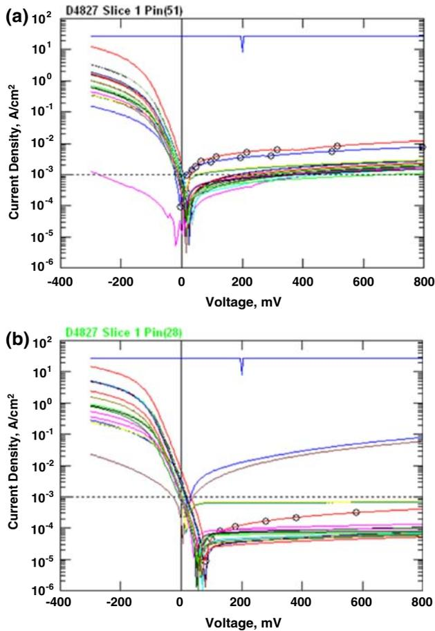
Fig. 3.  $I$ - $V$  curves of mini-arrays on test bar D4827.1 measured at 200 K. The mini-arrays have pitches ranging from 15  $\mu\text{m}$  to 40  $\mu\text{m}$ , and via diameters ranging from 4  $\mu\text{m}$  to 10  $\mu\text{m}$ . (a)  $I$ - $V$  curves prior to decomplexing bake. (b) After decomplexing bake at 120°C.
