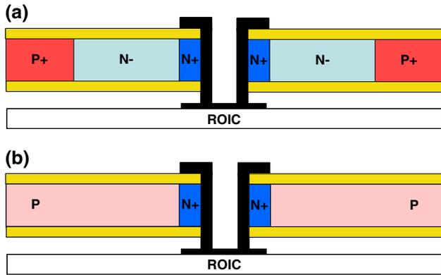
Fig. 1. Schematic cross-sections through a HDVIP diodes. (a) Conventional diode architecture. (b) HOT architecture.
