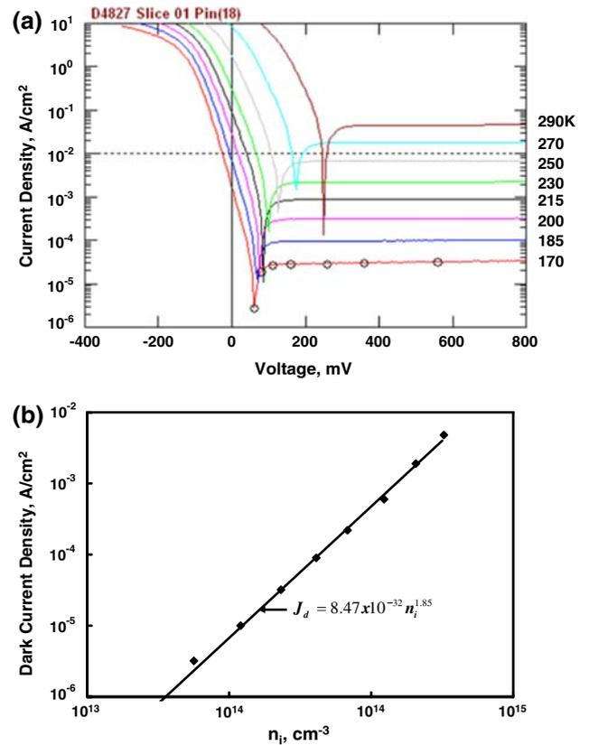
Fig. 4. Dark current density in a 30- $\mu\text{m}$ -pitch 10- $\mu\text{m}$ -via mini-array on test bar D4827.1 at various temperatures. This test bar had a HgCdTe thickness of 2.34  $\mu\text{m}$  and a 77 K cutoff of 5.175  $\mu\text{m}$ , corresponding to a cutoff of 4.43  $\mu\text{m}$  at 250 K. (a)  $I$ - $V$  curves. (b) Dark current density versus intrinsic carrier concentration,  $n_i$ .
