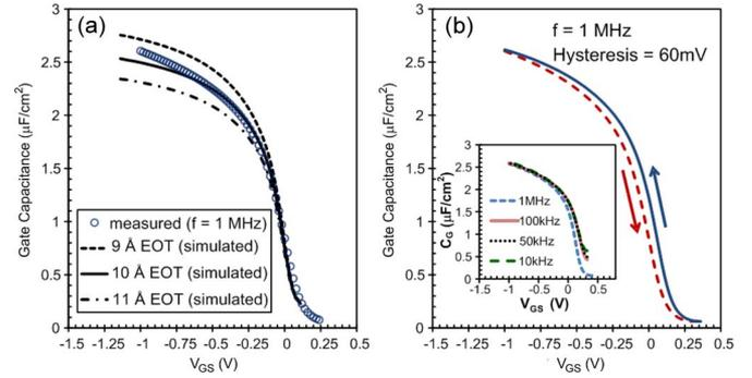
Fig. 3. (a) Measured gate-channel  $C$ – $V$  characteristics of s-Ge channel p-FETs; Overlaid are QM simulated  $C$ – $V$  curves for EOT = 9, 10, and 11 Å, demonstrating sub-1-nm EOT. (b) Hysteresis and frequency-dispersion  $C$ – $V$  characteristics of s-Ge p-FETs with XTEM shown in Fig. 1(b).
