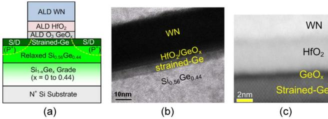
Fig. 1. (a) Structural schematic and corresponding cross-sectional (b) TEM and (c) high-resolution STEM images of the fabricated ultrathin s-Ge channel p-FETs with GeO<sub>x</sub>/HfO<sub>2</sub>/WN gate stack.
