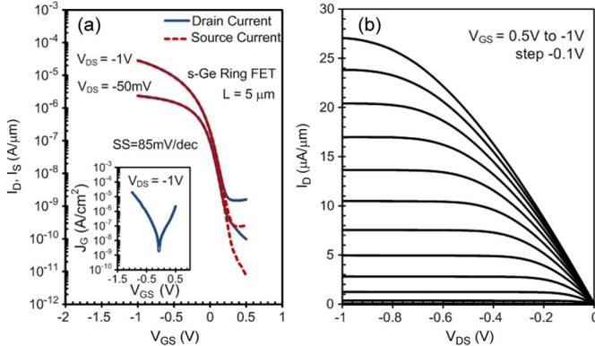
Fig. 2. Typical (a) transfer and (b) output characteristics of  $\sim 6$ -nm-thick s-Ge channel ring p-FETs ( $L = 5\ \mu\text{m}$ ) with GeO<sub>x</sub>/HfO<sub>2</sub>/WN gate stack. The inset of (a) shows the typical gate leakage characteristics.
