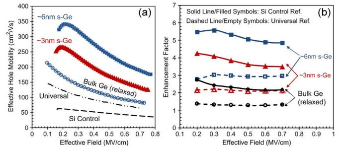
Fig. 4. (a) Effective hole mobility of  $\sim 6$ - and  $\sim 3$ -nm s-Ge channel p-FETs with HK/MG stack versus effective field. Overlaid are universal hole mobility, mobility of processed Si control, and bulk relaxed Ge [13] with O<sub>3</sub> surface passivation and HfO<sub>2</sub>/WN gate stack. (b) Corresponding mobility enhancement factor versus effective field over the (dashed line/empty symbols) universal and (solid line/field symbols) Si control.
